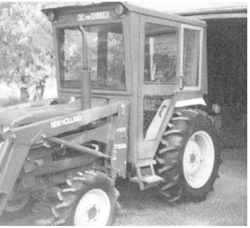
Van Valkenburg had the cab cut down 1 ft. to fit the New Holland tractor.
