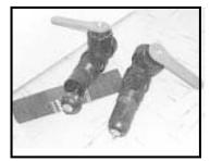
The 2 in. dia. valve is built out of polyethvlene and stainless steel.
