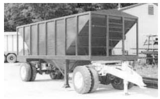
The 20 by 8-ft. wagon was built using the rear axle and jacks off a semi trailer and the front axle and fifth wheel dolly off a semi tractor.
