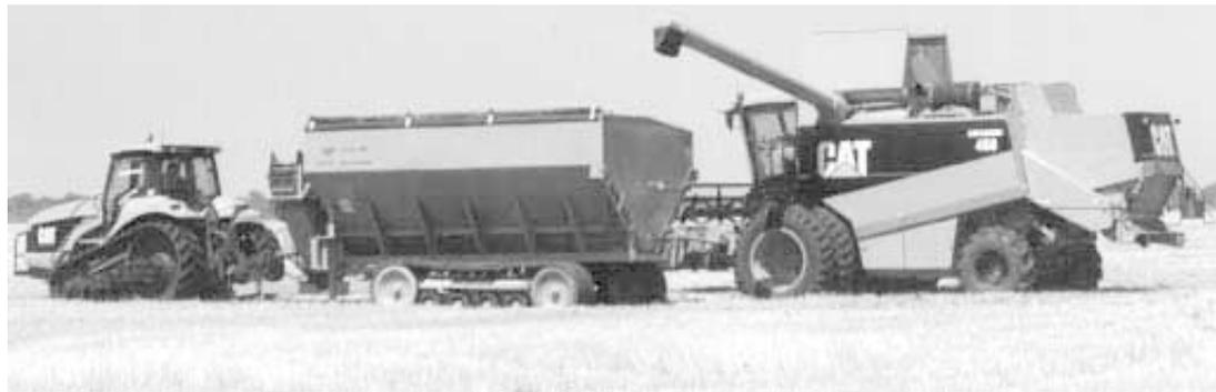
**New 1,000-bu. grain cart mounts on Caterpillar rubber tracks and is designed so that the Cat VFS 70 track system can be removed by pulling two pins and jacking up the wagon. Tracks can then be used on other equipment.**
