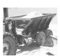
Machine discharges sand 3 to 15 ft. in either direction.
