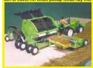
the bale chamber. After the 8-ft. long bale has been formed, a retractable knife cuts it in half. I'm now building a new working prototype which I think could increase the output even
