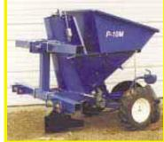
U.S. The 1 and 2-row planters are fully mounted and can be used on tractors with Cat. I or II hitches. Their light weight allows use of a smaller, more maneuverable tractor. The 2-row model adjusts to row spacings from 26 to 36 in. The low height of the 200-lb. capacity seed hopper makes it easy to load from the ground on a pickup bed.
