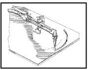
To make a circle, you stick the pointed end of the circle cutter into a dent made by a center punch.
