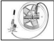
The "Round Again" wheel rim straightener is designed for heavy duty truck wheel rims, 17 though 24.5 in. It consists of two half round forms powered by a 10-ton ram. When pressure is applied to the hydraulic pump via a foot pump, the ram exerts pressure on the damaged area and returns it to its original shape.
