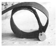
pin to join the two ends of the strap. It was sewn into the strap by a shoemaker. To use, he simply tightens the strap loop around the filter with a wrench, and keeps tightening until the filter works loose. Works great and never stretches out the way some commercial strap-type wrenches do.
