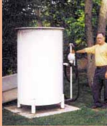
Kominek set this 200-gal. tank on end and made a floating cover out of wood covered with fibreglass-type resin. It covers the entire surface of the fuel to keep it from evaporating.
