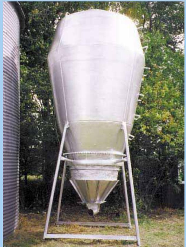
To make the feed bin, the Dewitz's removed the mixing chamber from an old cement mixing truck and mounted it upright on four legs. Steel ladder rungs were welded to one side to get up to the hatch on top.
