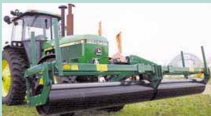
Roller mounts on front 3-pt. hitch and is available in 12 and 15-ft. widths.
