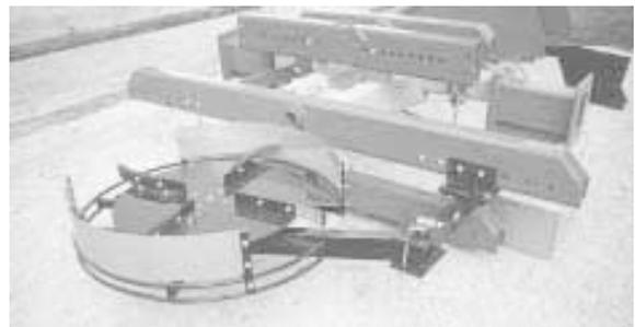
Hydraulic-driven spreader mounts on steel swing arm.
