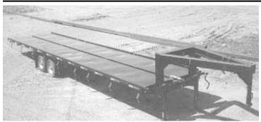
In this position, the trailer is a conventional 36-ft. long  $\overline{\text{flatbed.}}$
