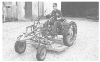
The biggest challenge in mounting the mower was adapting the vertical belt pulley on the tractor to the horizontal drive on the mower.
