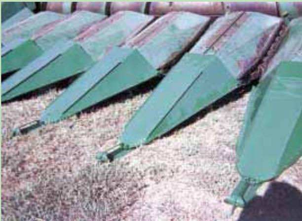
Floating header points bolt on in place of original points and are equipped with a steel shoe that's free to pivot up or down as it slides along ground.
