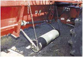
The 14-in. dia. rollers mount on steel arms that attach to header.
