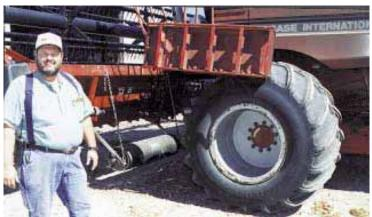
Grigsby uses 5-ft. wide "stalk rollers" on back of his 25-ft. grain platform as well as on his 8-row corn head. The rollers protect 50-in. wide "logger" flotation tires.
