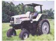
System increases ground clearance by holting heavy-duty drop final drives to tractor's rear axle housing.
