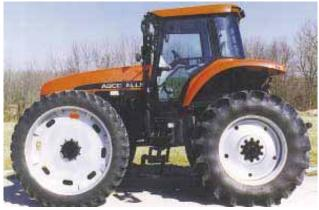
Agco 2 and 4-WD tractors up to 145 hp can be converted into high-clearance rigs for spraying and cultivating tall growing crops.
