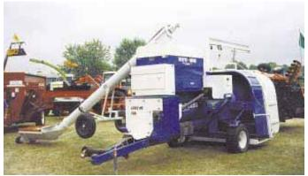
Roller mill mounts on top of bagger and is belt-driven off a pto shaft from bagger.
