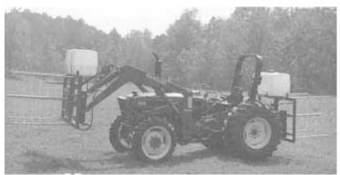
Tractor-mounted injection system uses 50-gal. reservoir and pto-powered roller pump to inject nutrients into bale. To use, you spear bale and then activate pump to treat it.
