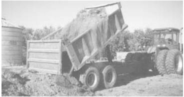
Steve and Joe Peters converted a mid-1970's Ford tandem axle, 13 cubic yard dump truck into this dump trailer. Tractor pto-drives truck's original hydraulic pump.
