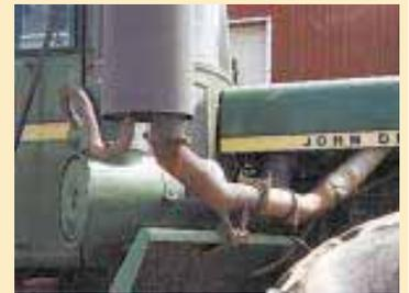
Muffler now mounts on a 90° exhaust elbow which Davis bought new from Deere.
