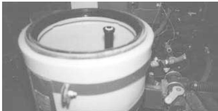
Leismeister screwed a pop-up sprinkler head inside the small induction tank on his Spray Air sprayer. He holds empty jugs over the head to rinse them out.
