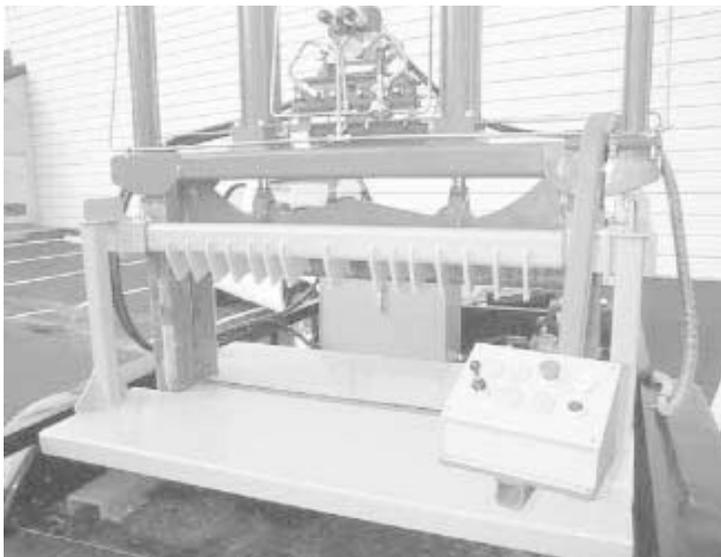
Machine has a long steel blade with hold-down bars on either side of it. Bars are lowered to grab each side of tire and bend it downward, stretching the rubber very tight so it's easier to cut. Blade is then lowered into tire.
