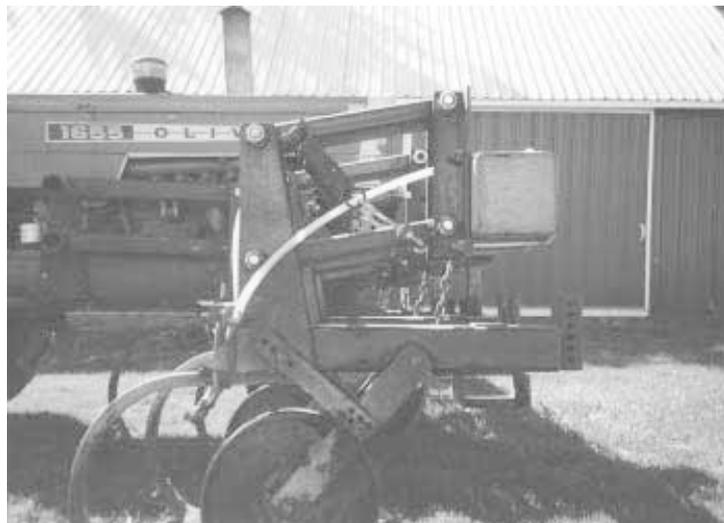
He cut the cultivator's 7 by 7-in. toolbar in half, then built a framework with parallel linkage to lift it with a hydraulic cylinder.
