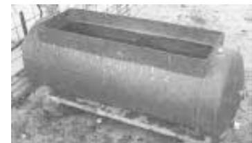
Seltzer made the cattle tank by welding two 40-gal. electric hot water heater tanks together end to end.
