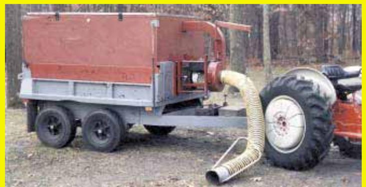
Trailer is equipped with a commercial leaf blower which pulls leaves through a 12-ft. long hose and into the box.
