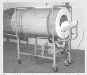
Vegetable washer works something like a cement mixer, with vegetables loaded into one end of barrel via a plastic chute.
