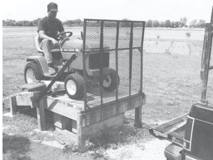
**Pivoting metal ramp lays down onto pickup tailgate for loading ATV. To make double use of ramp, Meffert built a dog house underneath.**
