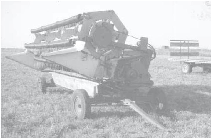
Wagon running gear was lengthened by 4 ft. A 1-ft. high wooden board keeps grain platform sicklebar from sagging.
