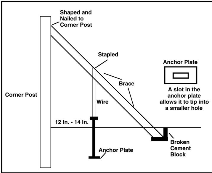
By installing an anchor that ties to the corner brace, you can keep posts from lifting out of the ground, says Myron Hebbert.
