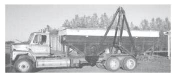
Tandem axle truck is equipped with two 325-bu. Unververth gravity boxes, as well as two drill fill augers.
