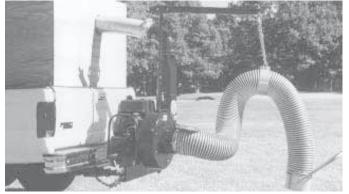
Leaf vacuum hooks up to receiver hitch. A 10-ft. long flexible hose sucks debris up into hopper on pickup bed. Suction fan is driven by its own auxilliary engine.
