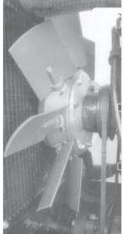
A small 12-volt air compressor is used to change angle on fan's blades by 90 degrees, allowing fan to blow out instead of suck
