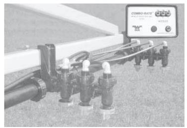
"Combo-Rate" uses multiple nozzle bodies that mount in-line at each nozzle location. Air-controlled shut-off valves turn nozzles on or off from cab.
