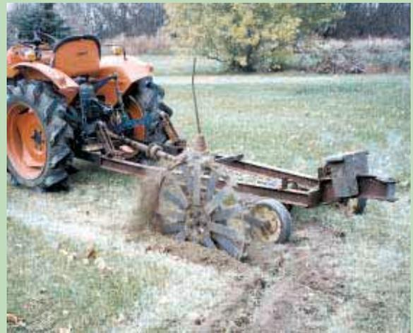
"My Kubota tractor goes so slow I can get off and clean up the trench on-the-go," says Del Bergeron about his home-built trencher. Trench is dug by an 18-in. dia. steel wheel.
