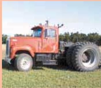
Truck-tractor's short wheelbase and individual air brakes make the tractor easy to maneuver on headlands, say Gerald and Glen Oetken.
