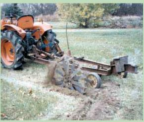
"My Kubota tractor goes so slow I can get off and clean up the trench on-the-go," says Del Bergeron about his home-built trencher. Trench is dug by an 18-in. dia. steel wheel.
