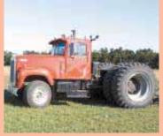
Truck-tractor's short wheelbase and individual air brakes make the tractor easy to maneuver on headlands, say Gerald and Glen Oetken.
