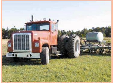
Oetken's powerful truck-tractor cost a total of just \$12,000 to construct. The IH semi's original twin-screw axles were replaced with a 100-ton Euclid rear end.
