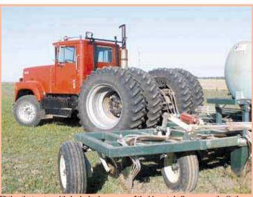
Fitting the tractor with dual wheels was one of the biggest challenges, say the Oetkens. They made wheel spacers out of 30-in. dia. natural gas pipe.
