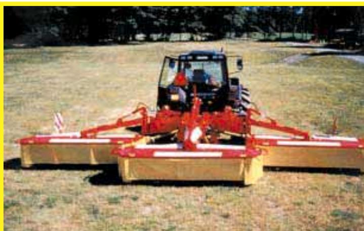
Pottinger Multicat 9000 is fitted with three 10-ft. sections of disc mowers and drum-type conditioners. All three sections can be mounted on back of a bi-directional tractor.
