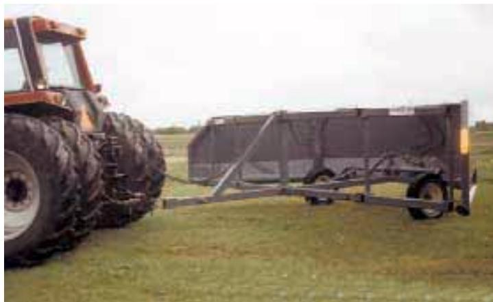
A pair of baffles, one on each side, close off ends of the 25-ft. wide drag.
