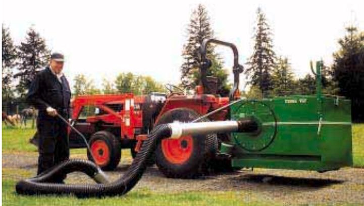
Pasture vacuum has a 22-in. impeller which provides enough suction to pick up manure, even in thick grass, and mulch it before blowing it into a hopper.
