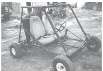
This heavy-built 6 1/2-ft. long, 74-in. wide go-cart is equipped with two bucket seats out of a Ford pickup, allowing it to comfortably seat two adults.
