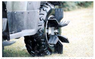
Mud paddles attach to a rim that fits tightly inside wheel rim. Paddles pull through mud and snow but are out of the way on dry ground.
