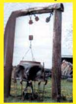
cut off the top bead and then pulled the tractor rim up through the tire using a winch mounted on the back of my homebuilt 4-WD tractor. The tire is held to the ground by the hold-down hooks that are anchored to the ground.
