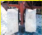
of conduit into a semi circle shape and bolted it to the underside of the belting. We also bolted a short length of steel shaft to each conduit. The next step was to U-clamp a pair of 8-in. long steel shafts onto the axle. The short length of shaft on each fender slides over the top of the axle-mounted shaft and is held secure by a set screw. That makes it easy to take them off when we park it so cattle won't rub on them. (Denny Dodd, 20093 T Ave., Reinbeck, Iowa 50669 ph 319 989-2591)
