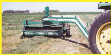
Last year FARM SHOW published an article on our add-on conditioning rollers designed to crush hay stems to cut drying time in half (Vol. 23, No. 2). The rollers are designed to replace rollers on most models of swathers and mower-conditioners. However, they don't fit all models. To meet the need we've just introduced our own 8-ft. pull-type conditioner as a stand-alone unit. The PT 8000 is designed as a followup conditioning system for use behind your swather or mower.
