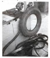
We're excited about our new tire cutting machine that cuts both steel-belted radials and bias ply tires into 2-in, wide strips that make great fencing material. We make a variety of other tire cutting equipment, which has been featured in FARM SHOW, but this is the first time we have built a machine to cut up steel-belted radials. In this area of the country you can get as much as \$2 apiece to
