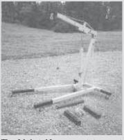
They fabricated four new parts to convert the rolling engine hoist into a 3-pt. mounted crane.
