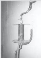
Air hose runs through hole cut into side of pipe and up to quick coupler.
