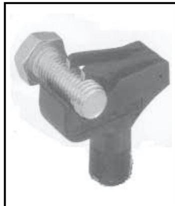
**Two hardened steel blade on restorer head are guided by undamaged thread to regroove damaged areas.**
