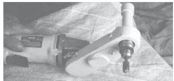
Belt-driven extension for chop saw can also be used to power a drill chuck.
