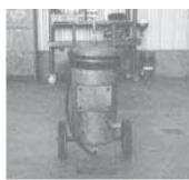
Air pressure pumps oil out of tank.
