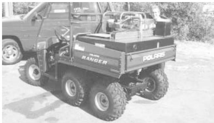
CFX Fast Attack ATEV (all terrain emergency vehicle) mounts on a Polaris ATV. Its pumping unit can move about 100 gal. of water per minute.
