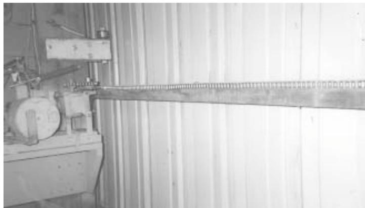
Automatic opener was made from a 1/3 hp motor salvaged from a garage door opener. It opens the 16-ft. door on Brandenburg's shop.
