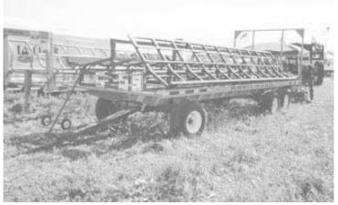
Carrier is equipped with two cradles and unloads one side at a time without the use of hydraulics, chains, or motors. The operator simply turns a crank to trip the cradles.
