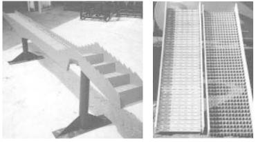
Straw walker bolts on in place of combine's original walker and can be completely closed off or opened to 80 percent. Size of openings is adjusted by using a lever. Photo at left shows entire assembly. Photo on right shows walker open and closed.
