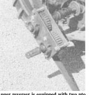
Auger reverser is equipped with two pto shafts - one that hooks to tractor pto and another that drives the auger.
