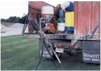
Ladder mounts at right angle to back of truck, making it easy to climb in.
