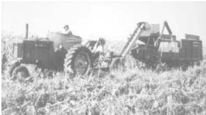
conventional flat bed box wagon. The wagon is equipped with a hydraulic dump for putting corn into a bin.
