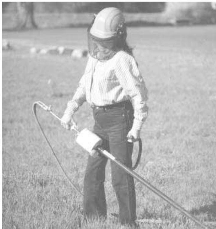
Underground blaster uses an electronic solid state ignition system powered by two 9-volt batteries. When you inject gas into the tunnel there's a 1 1/2-second ignition delay.
