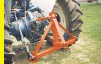
of tubing on top and braced it up real well with 1/2-in. flat stock. I bought a pair of 1 1/8 in. threaded pins for the drawbar pins. I cut a hole in the bottom so if I ever break a pin I could change it. It gave me a rugged hitch that will last a lifetime. I can insert a variety of hitches. It will even take a pintle hook. **(Basil L. Powers, General Delivery, Stratton, Maine 04982 ph 207 246-3092)**
