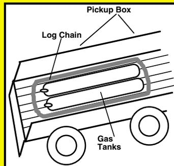
To keep compressed gas tanks from rolling around in the back of my pickup, I
