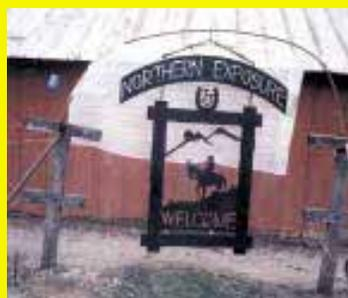
stead sign that would last. He drew the design with soapstone on a 3 by 4-ft. sheet of 12-ga. metal. He then cut it out with a plasma cutter. The result is eye-catching and durable. He cut the name - Northern Exposure - out of a sheet of 10-ga. steel and mounted it on top. **(Michael Zinghiem, 5501 Boxelder Rd., Marshall, Wis. 53559 ph 608 655-3530)**
