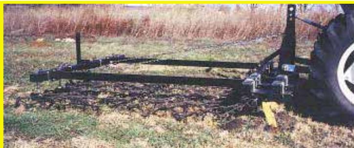
Anyone with livestock on pasture should take a look at our new B-33 Mole renovator attachment for running ahead of our MultiFlex heavy-duty 3-pt. pasture harrows. The mole renovator loosens compacted soil to a depth of 4 to 6 in., allowing water and air to soak into the soil upon contact. It reduces runoff. The harrow behind mixes residue with surface soil. The mole knife does not disturb the surface, so you can broadcast seed before running the harrow equipped with the mole knives.
