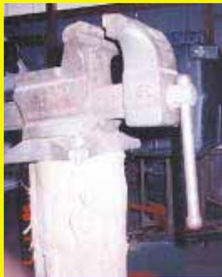
large wooden fence post sunk in the floor of my shop so I can move all the way around it to get the best angle for whatever job I'm doing. I set the post securely in the floor, then bolted the vise to it.
