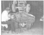
An eye bolt is permanently installed in the front end of the Cub Cadet. I attach that to an overhead chain hoist and lift. Once the tractor is up, I put a safety stand under the deck and lock the rear wheels to keep the tractor from moving once it's raised. I use a small 4 1/2-in. hand grinder, which I bought out of a mail order catalog, to sharpen the blades. This method is much quicker and easier than detaching the deck."
