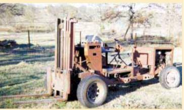
To see the rear-mounted forklift, Eddings moved the seat, steering wheel and controls 90 degrees to the right, so driver faces passenger side.
