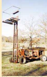
Eddings started with a late 1970's Chevy Luv 4-WD pickup and mounted a 3-stage forklift mast on it. "The mast lifts 12 ft. high," he says.
