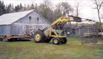
Chain harrow hangs from front-end loader during transport.
