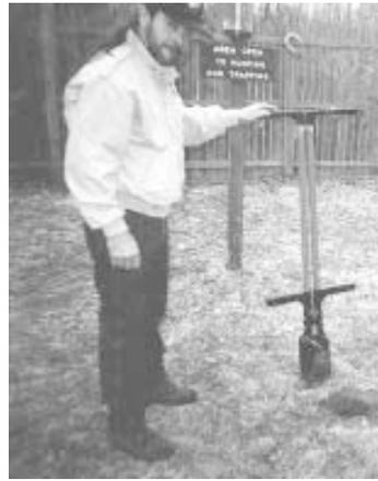
Post hole digger is equipped with foot rests that you jump onto.
