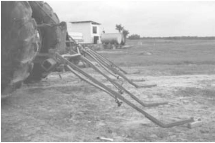
Sprayer is built on a tractor-mounted toolbar, with "legs" that angle back toward the ground at a 45 degree angle.
