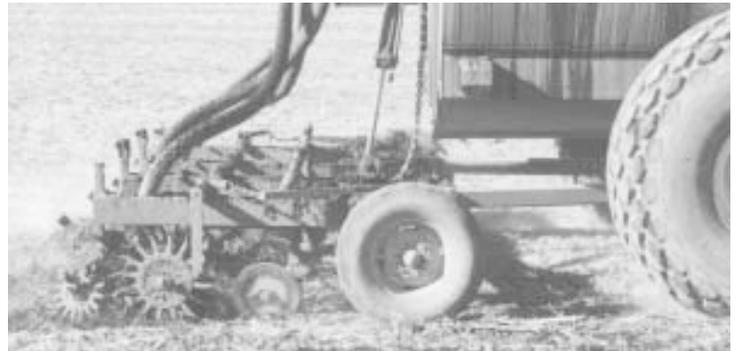
Rotary hoe wheels on new injector prevent it from plowing up slabs of soil.
