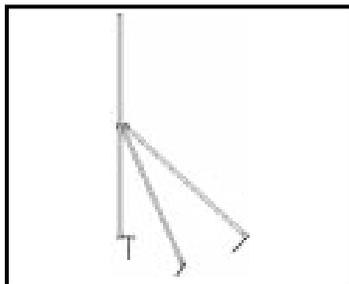
**Tripod corner post has a solid steel spike which can be stepped in or driven into ground. Free-swinging braces are attached about half way up the post.**
