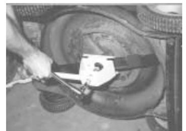
Tool fits over blade and is held in place by tabs on either side.
