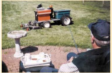
Godfrey installed model airplane remote control servos on the mower to turn its motors on and off. He uses a joystick to steer the machine.
