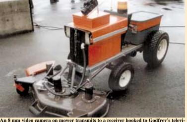
An 8 mm video camera on mower transmits to a receiver hooked to Godfrey's television set.
