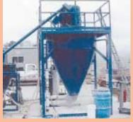
Vortex machine (above) can be used to process all kinds of products for waste disposal or for use as feed ingredients. It reduces virtually any product to dust including chicken feathers (above right), broccoli (right), chicken gizzards (below right), and tin cans (below).
