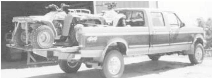
When inserted into a pickup receiver hitch, the steel rack holds at least half the weight of a 4-wheeler.
